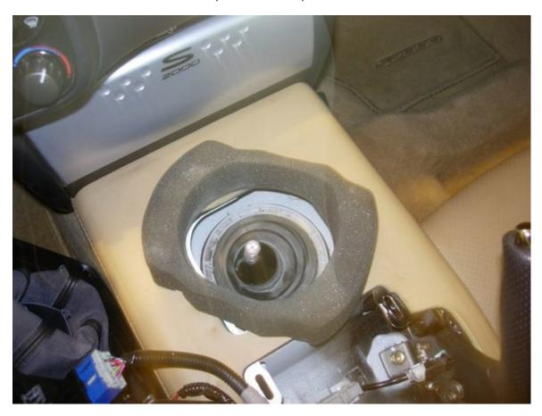
Now for the second hardest part of this process - getting the rubber shifter boot off. Its held on with a plastic ring with four clips at each corner - there are little arrows on the ring that show you where they are. You need to use a flathead screwdriver to pry them off from inside the ring. Major PITA and I still managed to break two of the clips getting it off for some reason.
