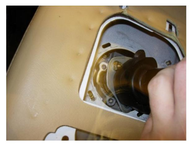
Once you get one bolt in to keep the shifter from springing up, insert the other two and keep realigning the bolt plate. Once all three are in, tighten them down. Test the shifter and make sure you can get into gears! If all is good reapply the rubber seal over the three bolts.
