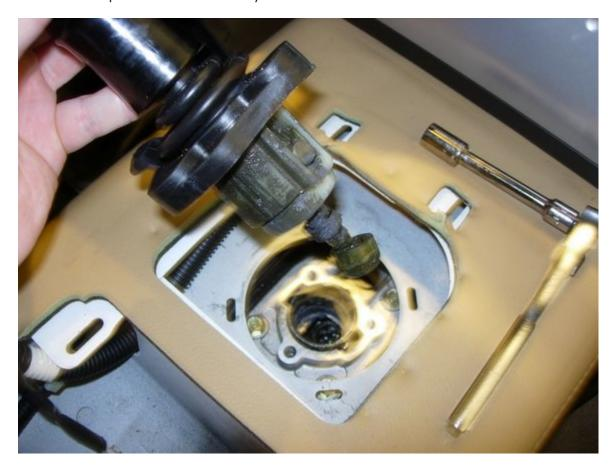
Pull the shifter out, be mindful of the spring - it may stay in the hole, or come with the shifter, but its covered in grease, so don't let it drop in the car!
