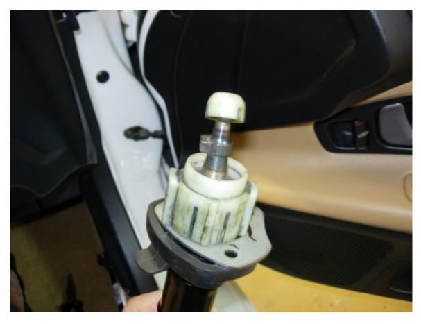
Grab the Urea grease and start greasing - get as much as you can in the shifter assembly, under the bolt
