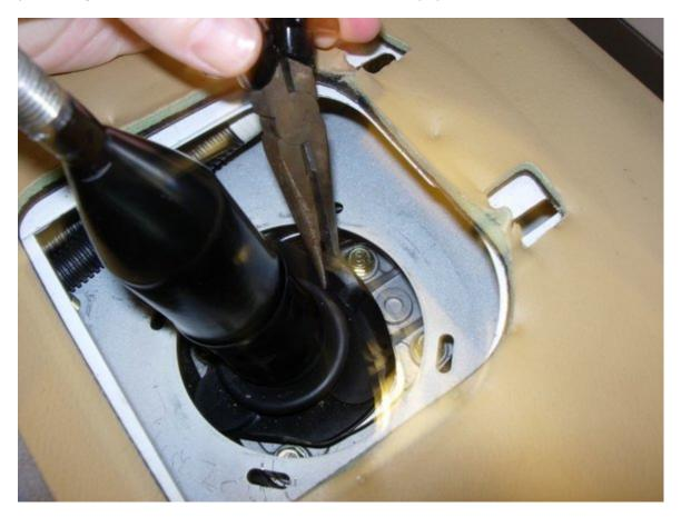
Now you can access the three 10mm bolts and loosen them. Note that the shifter is spring loaded, so it will pop a bit when you get the last one off. The bolt closest to the steering wheel seems to do the most to hold the shifter in place - I recommend you remove that bolt last.
