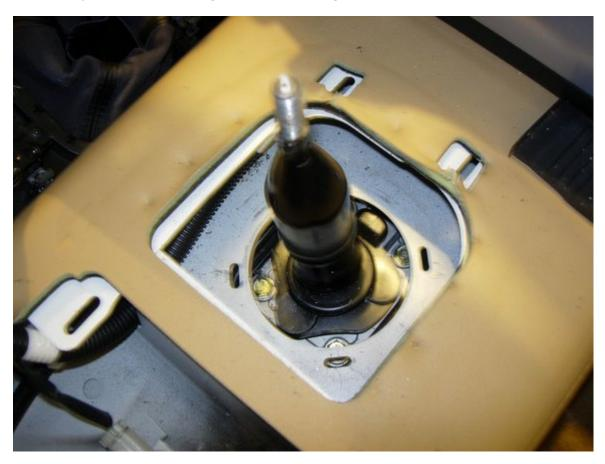
Now you'll see where the shifter is bolted to the car, under the rubber protective cover. Use needle nose pliers to grab the tab toward the front of the car and pop it off.
