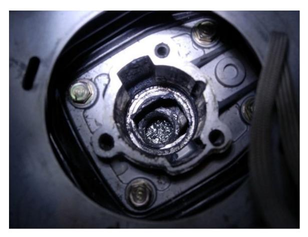
The shifter, quickly cleaned up. You can be more thorough with solvent, but I just wanted to get fresh grease in so I just got what I could with a rag. Inspect the ball cap for any cracks or chips - if its bad, replace it. Pivot ball at the end of the shifter = 54111-52A-003 COVER, PIVOT \$2.02
