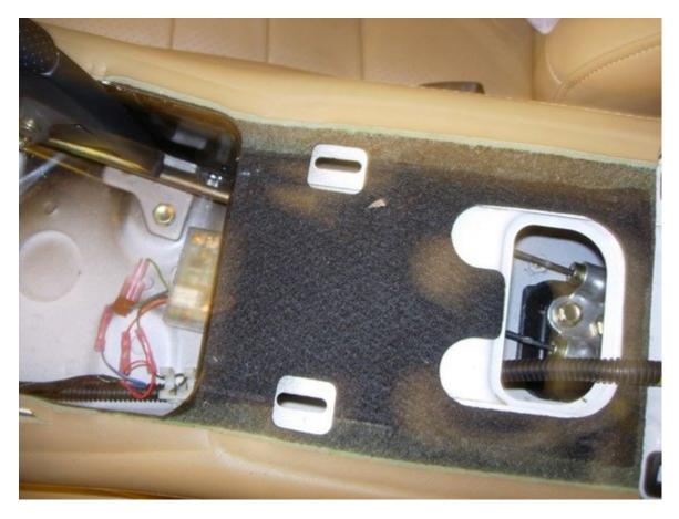
Pull the console up and over the emergency brake - the higher you can get the brake, the easier this is. You can disconnect the wiring harness to completely remove the center console, or just lay it over on the driver's seat so its out of the way.
