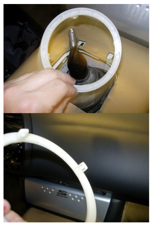
Once you snap the ring loose at all four corners, just lift it out, and then pull the rubber boot up and off the shifter. If you need a new ring - it's "Plastic Ring = 54107-S2A-003 HOLDER B, CHANGE BOOT \$2.68"
